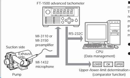
The number of pump revolutions is easily measured by monitoring exhaust noise. The rotational shaft in pump equipment is generally not exposed externally, making it difficult to perform measurement of revolutions based on the ordinary pulse detection system. In this example, changes in exhaust pressure are detected for revolution measurement with a microphone.
