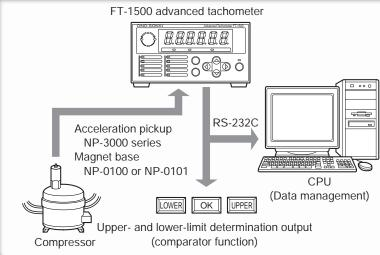
■ This is used for compressors that function as essential components of household refrigerators, vending machines, display cases, and air conditioning units. The number of revolutions of a compressor whose rotational shaft is not directly accessible is easily measured by combining the FT-1500 with an acceleration pickup.
